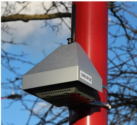
Particles are counted and allocated to sized bins. Any further calculations of mass – and there is considerable scope to use these in combination with on-board temperature, pressure and RH measurements – are based on this. At this point the AQMesh OPC faces
