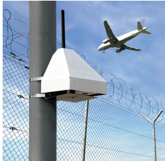
previous NO<sub>2</sub> sensors having a massive O<sub>3</sub> cross-gas effect (AQMesh v3.0 processing), we have made huge strides since then, particularly focusing on the key gas - NO<sub>2</sub>. AQMesh v4.0 NO<sub>2</sub> processing reliably delivers an R<sup>2</sup> of >0.6 in temperatures up to ~25 °C. The new v4.1 and v4.2 processing successfully tackles even higher temperature locations.
