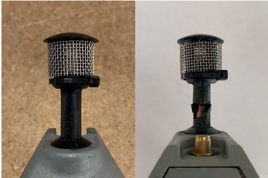
Good particle inlet - replace the collar
